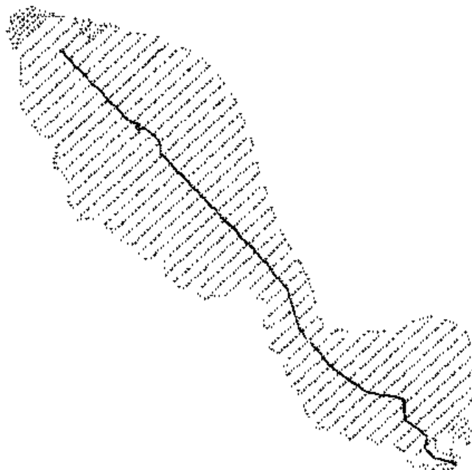
Figure 120. FINNMAP Tonle Sap Lake bathymetric survey in 1998 showing survey points.
