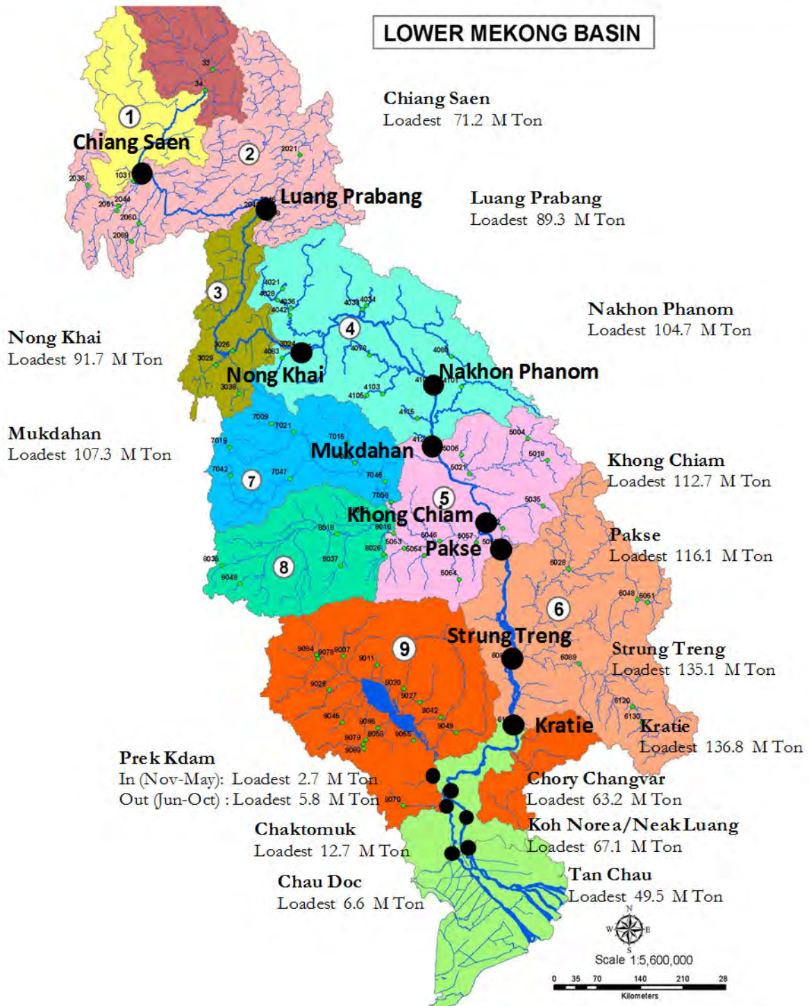
Figure 5-3 Summary of Analysis of Sediment Data to Annual Loads (Million Tonnes/yr) for Key Gauge Stations in the LMB
