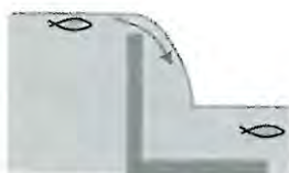
Overshot flood gates
